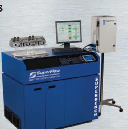
Additionally, the automated testing eliminates operator induced variables making the SuperBench extremely repeatable and accurate. It can test up to 240 hp (179 kW) per cylinder at test pressures up to 65" (165 cm) of water. The unique variable flow orifice adjusts flow range between 25 cfm and 1,000 cfm (12 - 472 l/s), based on computer input, to fit the valve size or valve lift.
