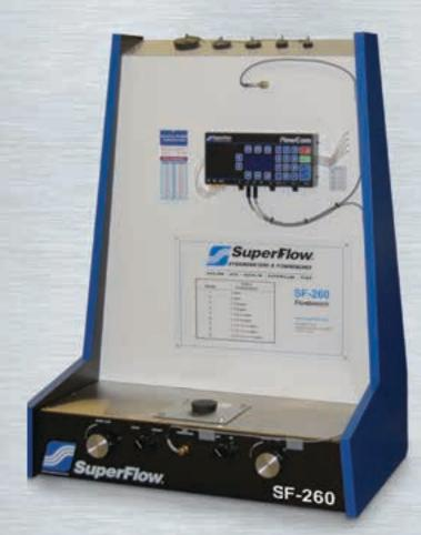
manometer type benches that require users to make calculations to achieve corrected flow numbers. The included automatic motor controller maintains constant test pressure without the use of knobs and valves and it also helps extend motor life by reducing heat generated during operation. Reduced heat means that operators can run the SF-260 for longer durations than benches lacking the motor control feature.
