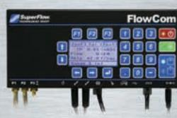
FlowCom<sup>™</sup> Air Flow Measurement Computer\* for rapid, accurate testing. This highly accurate, easy-to-use digital airflow measurement system gauges test pressure and temperature measurement to within 0.5° F. FlowCom<sup>™</sup> measures and calculates airflow in CFM. It has inputs for optional external devices like swirl meters, tumble meters and velocity probes. \*Standard on 260, 450, 750, 1020
