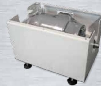
The AC Motoring Cube brings emissions level test data the CycleDyn. It allows you to perform R&D economically prior to final certification. The AC cube will simulate inertia, rolling losses and aerodynamic effects with the help of an advanced motor controller and WinDyn. Perform coast downs and evaluate parasitic losses or use SuperFlow's drivers trace software to perform emissions drive cycles.
