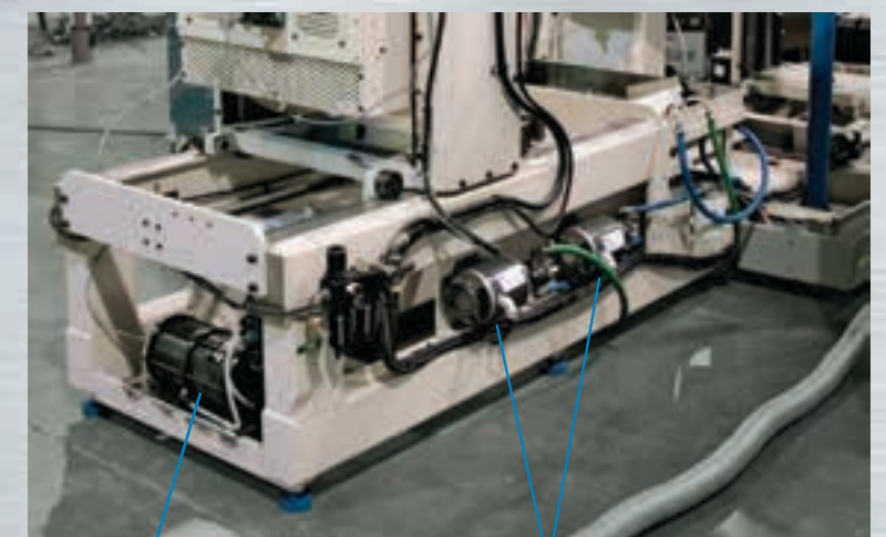
Air/oil booster for stall brake and linear adjustment.
