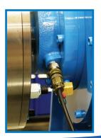
The following will confirm speed sensor wiring is damaged. The sensor cable connector will have two or three female plugs labeled "A" thru "C". Number of plugs is dependent on the type of speed sensor, engine dynamometers typically use a two wire speed sensor, while other Power Test/AIDCO products normally use a three wire speed sensor.
