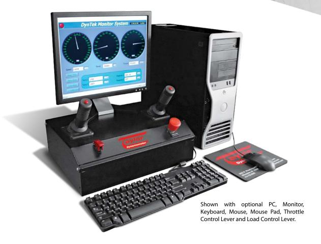
The DynTek-PC 2+2 engine dynamometer instrumentation system is a display only system intended for the most basic engine dynamometer testing requirements. This system provides for the measurement of torque in either tension or compression (both clockwise and counter-clockwise engine rotation), speed from a standard Magnetic Pickup along with two pressure and two temperature measurements.
