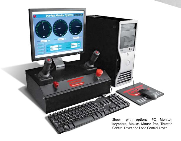
The DynTek-PC engine dynamometer instrumentation system is a display only system intended for basic engine dynamometer testing requirements. This system provides for the measurement of torque in either tension or compression (both clockwise and counter-clockwise engine rotation) and speed from a standard Magnetic Pickup. The system is designed to set on a table or desktop near the PC.
