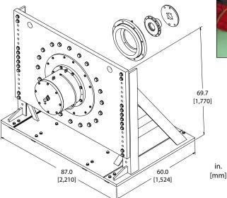
The 797 haul truck powertrain requires extensive custom tooling to test on the Hydraulic Test Center (HTC). This package provides all the custom tooling that is required for 797 testing except for tooling that is common to other powertrain testing. Additional accessories that are required for testing include: Instrumentation Package and Port for Worktable. Particle count testing can be performed with the purchase of Contamination Monitoring Accessory.
