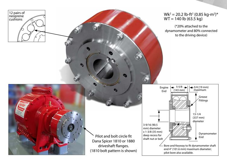
The Torsional Resilient Coupling is a dynamometer mounted coupling designed for use on our DX Series of engine dynamometers. The Coupling is intended to isolate the larger engine dynamometer from the high-amplitude torsional vibration of some smaller diesel engines with lightweight flywheels. The Torsional Resilient Coupling extends drivetrain life by diminishing or dampening vibration amplitudes over the operating speed range common to diesel engines.
