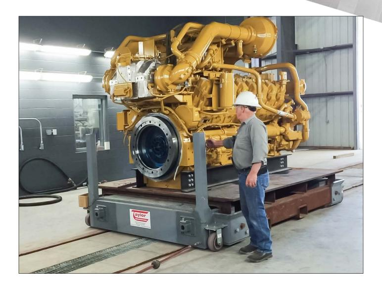
The 70,000 lb Engine Cart System is engineered to provide a moveable, durable and easy-to-use method of engine mounting for dynamometer testing. The Engine Cart System is designed for use on railroad type rails. Dead weight capacity is 70,000 lb (31,751 kg).
