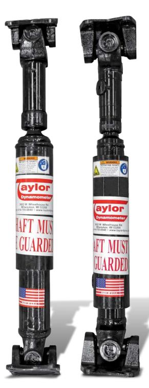
Vibration Dampening Driveshafts provide protection from system-destroying resonant frequencies by isolating the engine and the dynamometer. If the system is allowed to operate at resonance, the vibrations can quickly destroy bearings, bolted joints, instruments, mounts, or other associated equipment, as well as the driveshaft, dynamometer and engine. This energy, which otherwise could destroy system components, is absorbed by the Vibration Dampening Driveshaft.
