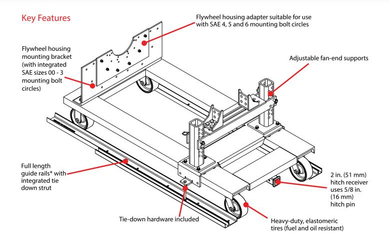
\*Mounting hardware not included 1/2 in. (13 mm) 3,000 lb (13 kN) pull-out strength floor anchors are recommended
