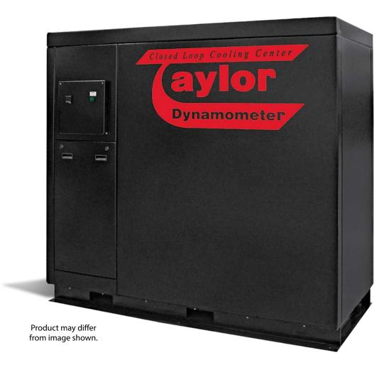
Taylor has a family of Closed Loop Cooling Centers (CLCC), each sized to handle the heat rejection typically required for engines that are of 1,250 hp, 2,500 hp, 4,250 hp, and 8,000 hp (932 kW, 1,864 kW, 3,169 kW and 5,965 kW). The CLCC allows you to use a glycol-based coolant to regulate an engine coolant circuit temperature while cooling the CLCC with the facility process water.
