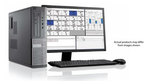
PowerNetTD is designed to provide a comprehensive, easy to use data acquisition and control system. PowerNetTD utilizes a Windows-based computerized data acquisition system to monitor and record speeds, torque, pressures, temperatures, flow rates and shift events.
