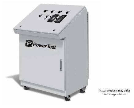
The ESC-Electronic Shift Console is the latest development for controlling transmissions when used in conjunction with a transmission test stand.
