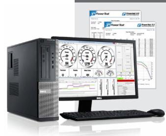
PowerNetTD is designed to provide a comprehensive, easy to use data acquisition and control system. PowerNet TD utilizes a Windows-based computerized data acquisition system to monitor and record speeds, torque, pressures, temperatures, flow rates and shift events.
