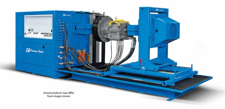
The 550E Test Stand is designed to test a wide variety of on-highway and off-highway, medium and heavy duty transmissions and torque converters. The machine accommodates mechanical and hydrostatic transmission testing with the ability to mount all standard drop-box or offset, engine, mid-ship and remote mounted powertrain systems.
