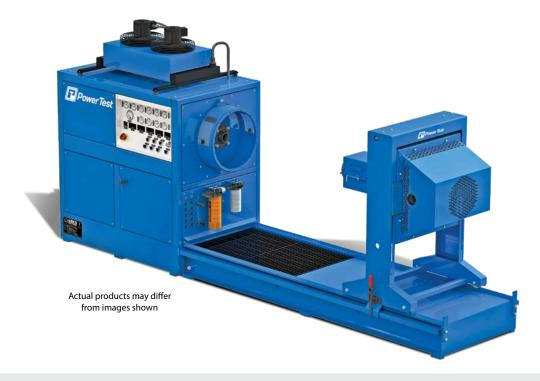
The 450E is designed for testing automatic and power shift transmissions used in commercial applications built by most popular OEM transmission manufacturers. This quiet, compact machine has been progressively engineered to facilitate quick transmission coupling and alignment. The 450E will perform the diagnostic tests to evaluate performance and troubleshoot faults.
