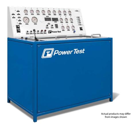
Because it can simulate actual operating conditions, the 265 Valve Body and Governor Test Stand performs with exceptional accuracy. A wide variety of operating conditions are created by combining electronic shift control components, shift selector and modulator controls, hydraulic oil pressure and motorized rotation for the governor. Using these controls, shift schedules can be customized to provide optimum transmission performance in every application.
