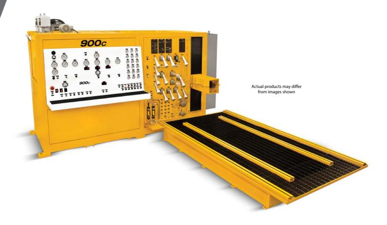
A versatile test stand designed for testing heavy-duty off-highway hydraulic components, the 900C Hydraulic Test Center features some of the most advanced technology on the market today. Designed for complete pump, motor, and hydrostatic transmission testing, the 900C is much more than a standard transmission test bench.
