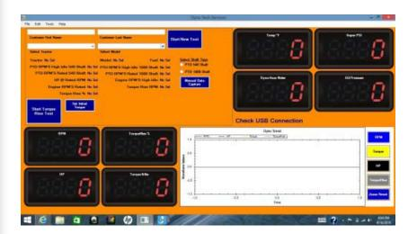
This system allows the operator to record the customer name, tractor brand, and tractor model. Once the brand and model have been selected the Power Pro 1000 will retrieve the Nebraska Tractor test specifications for engine and pto high idle rpm and rated rpm from the data file.
