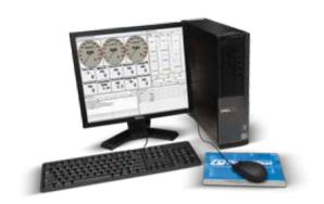
Through automated recording, verifiable test results are obtained and PowerNet TD assures that the data is true and accurate. Reports are easily produced that include your company logo, specific workshop information, customer information, and the manufacturer's specifications, along with the actual test results in table and graph formats. The paragraph feature allows you to enter any notes or observations made during the test.
