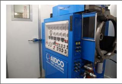
The operator can access the 450H and transmission being tested through the double hinged doors found on both sides of the container. Removable rails leading up to the dynamometer and a pulley and hoist system are used to bring the transmission into the container via our specially designed transmission cart. That same hoist is used to lift the transmission into place for installation to the test stand.
